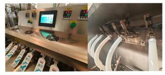
eliminating the disadvantages of low feeding efficiency and high air consumption of the plug pump. For difficult to seal formed bags, in addition to the traditional temperature control system, we have also added a time adjustment system. And the nozzle of the machine adopts a special design to ensure consistent sealing.
